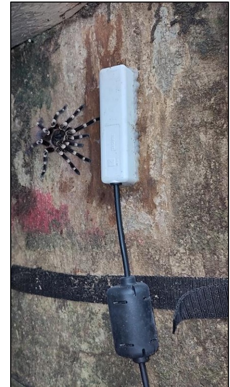
Scary spider + Teros 12 sensor to measure water content
